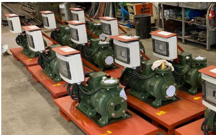
NR. 12 IR 50-200NA ITALY DUST SUPPRESSION DURING THE DEMOLITION OF "MORANDI" BRIDGE
